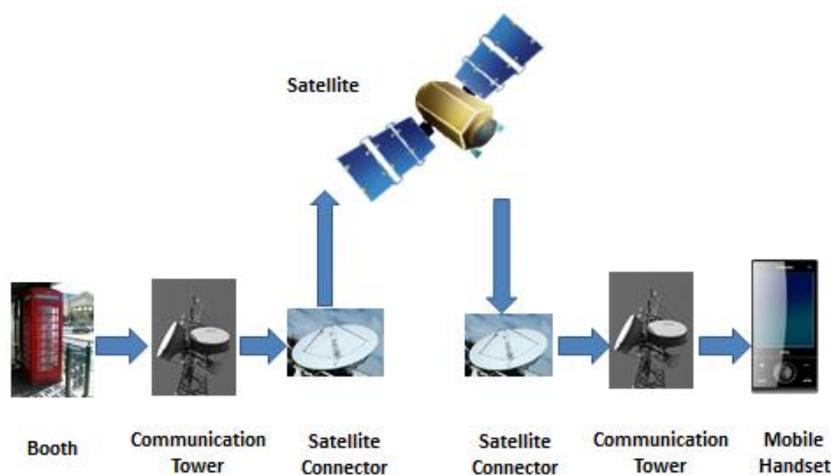
Figure 2.3.1: The process of telecommunication via handsets.
